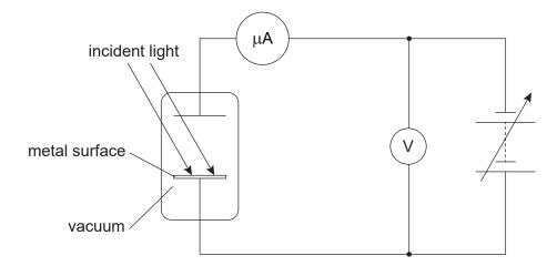
The work function of the metal surface is  $4.8\times10^{-20}\,J$ . What minimum voltage is required for the ammeter reading to fall to zero?
