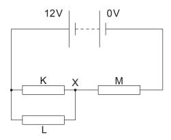
The resistor L is removed. What is the change in potential at X?
